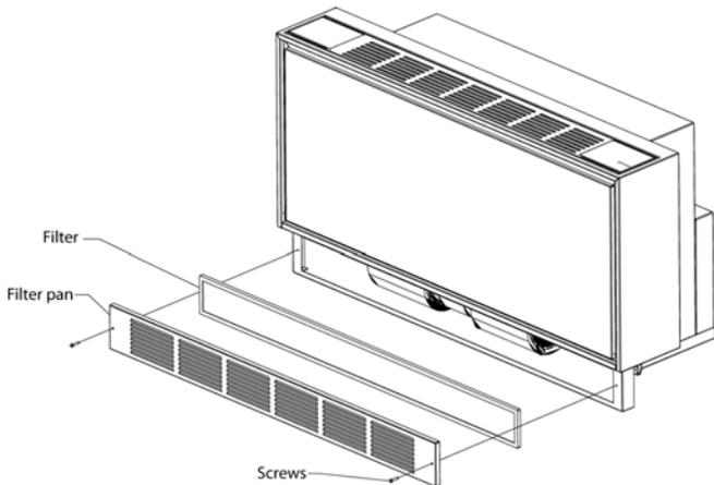
Remove two screws from the filter pan and remove. Lift filter out of filter pan and wash. After filter is dry place it back in filter pan and attach pan using the two screws. DO NOT run unit while filter is not installed.
