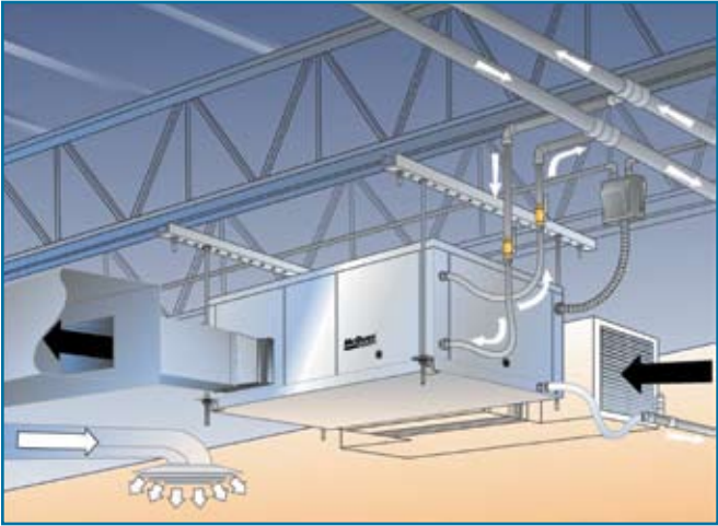
The 11.5" high cabinet of sizes 007, 009 and 012 allows greater design flexibility in applications with limited ceiling space.
