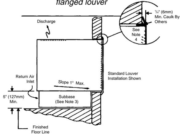
**Figure 9. Masonry construction, front inlet, stamped flanged louver**
