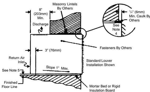
**Figure 10. Panel construction, bottom inlet, stamped flanged louver**
