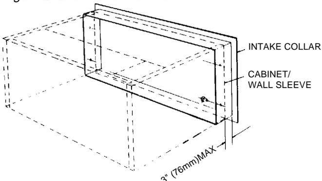
2. Place the louver frame in the wall opening from the exterior of the building, and apply firm pressure so that the caulked frame flanges are snug against the exterior of the building. Secure the louver frame to the wall if desired.
