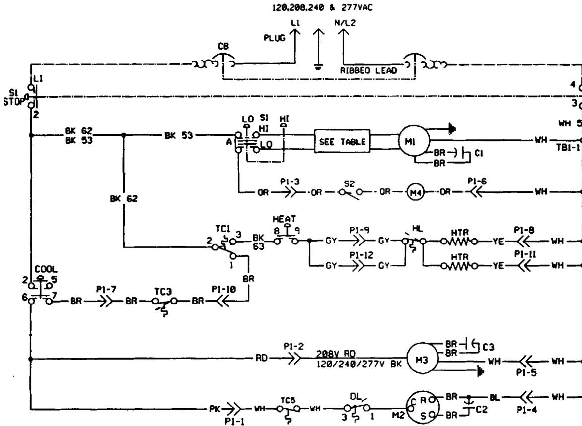
Figure 27. Enersaver heat pump with unit mounted thermostat, electric heat, no setback, manual change over
