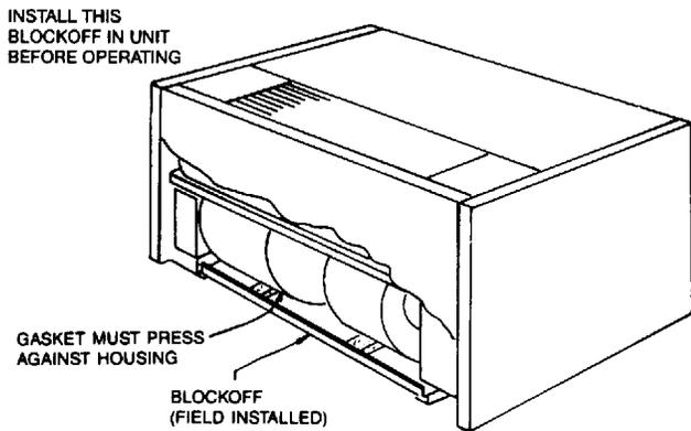
Figure 17. Front inlet block off detail
