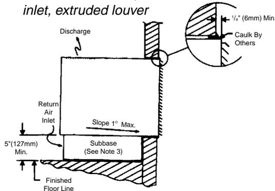
**Figure 8. Masonry construction, bottom inlet, extruded louver**
