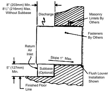
**Figure 9. Masonry construction, front inlet, extruded louver**
